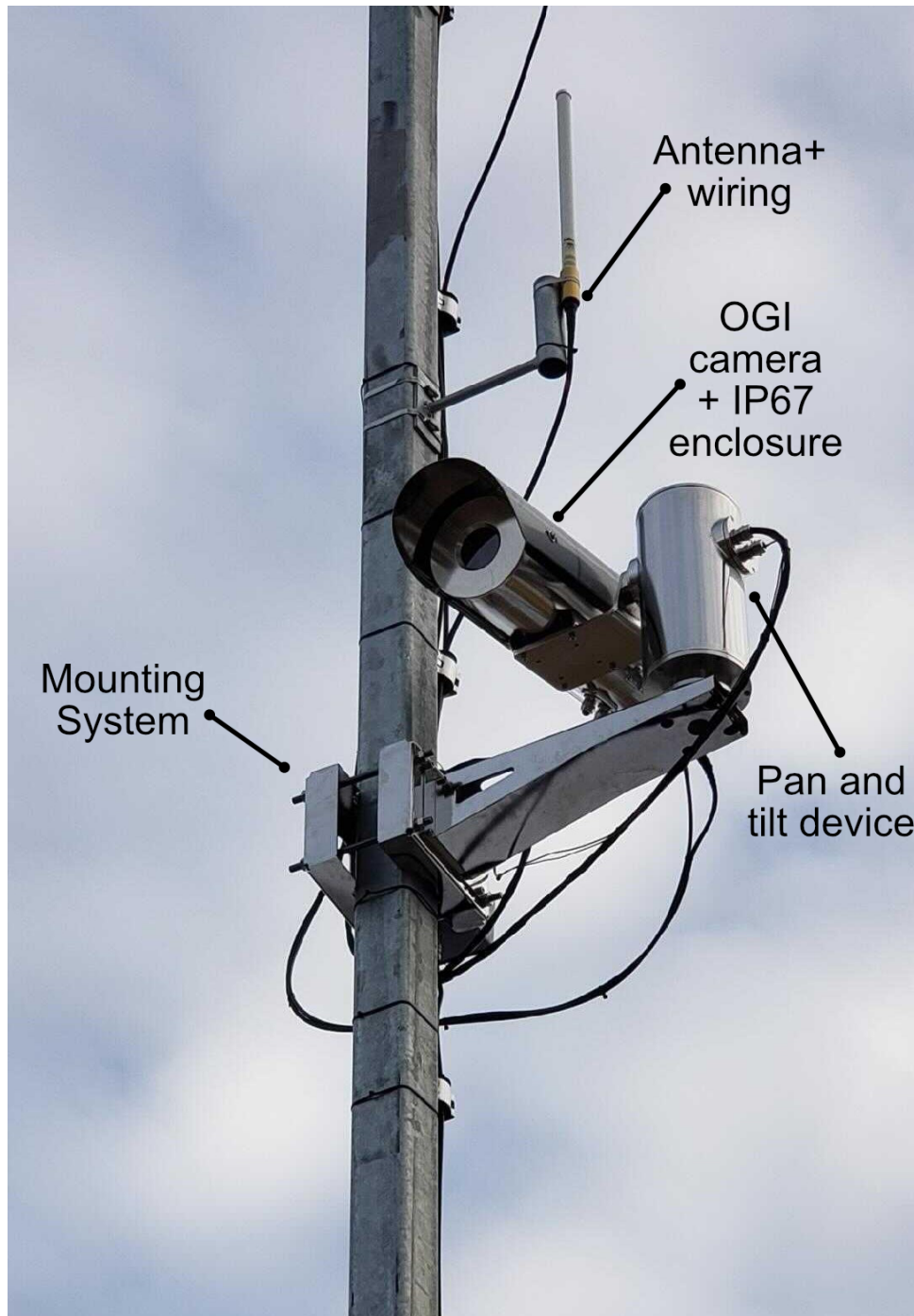
Figure 2: The Clean Connect OGI camera
